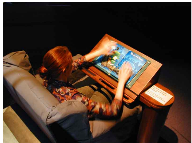
Fig. 1. The Listen Reader provides a classic immersive reading environment: a comfortable chair, a polished hardwood reading stand, and beautiful paper pages in a soft leather book binder. High-quality embedded audio and responsive proximity ("magic") sensors add to the sense of immersion.
