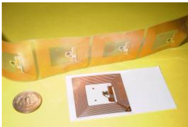
Fig. 2. RFID transponders (tags). Flexible copper printed onto clear plastic, embedded between two printed sheets to create one page thickness for the Listen Reader books. Each transponder has a unique ID. As of September 2000, tags about half this size are available.
