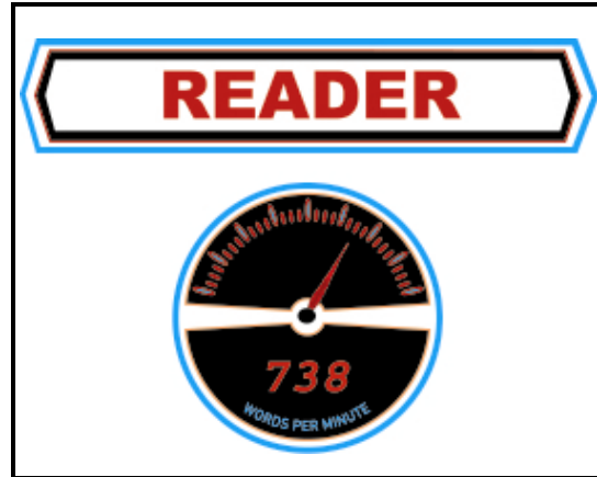
Figure 2. Presentation graphics and physical overlay for Speeder Reader . Blue indicates the side-lit lasercut Lexan overlay; red and black, and the background to the text, are all screen display areas; white shows where physical layers of felt and black plastic (under the top-layer Lexan) block the rest of the computer monitor from view.
